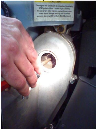
6. Once the shaft is out, leave the removal tool that was used in the gear so it doesn't fall doesn't fall in chain case.
