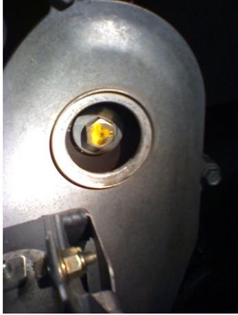
4. Apply brake and remove the bolt/washer from top gear (16mm). Be careful not to drop the bolt/washer in the chain case
