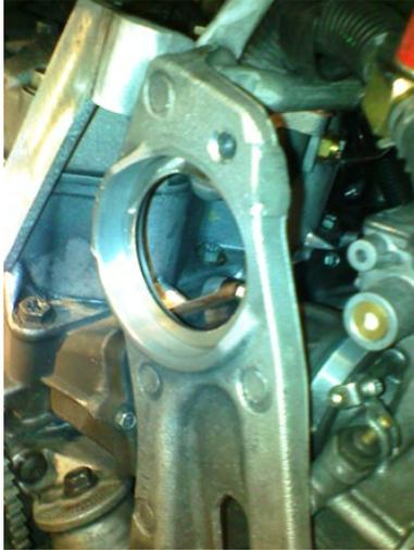
9. Install jackshaft. Once near the gear, lift the holding tool to align spline. Reinstall bolt/washer with red Loctite with 26 ft-LBS. Install black plug. Tighten chain case.
